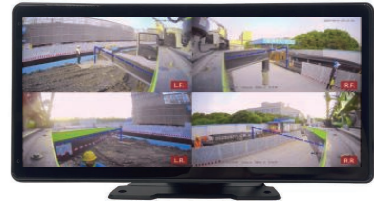
The auxiliary lines indicate the positions where the outriggers will reach when they are fully unfolded
