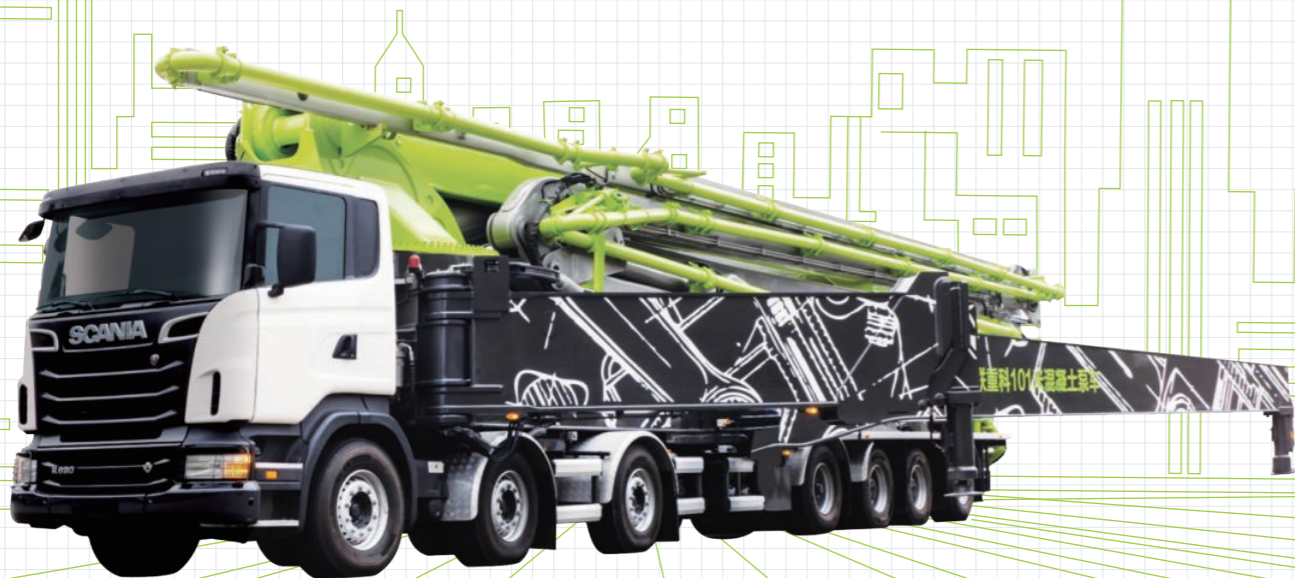
101 truck-mounted concrete pump
